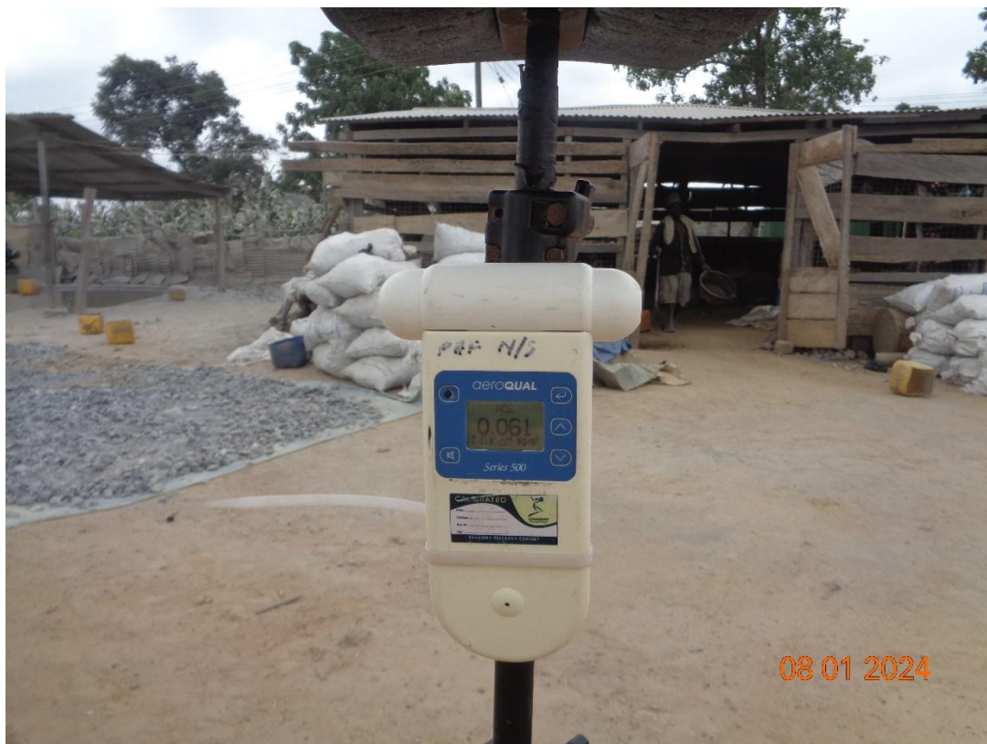
Plate 3: The Aeroqual Series 500 Gas Monitor Deployed at AN4 (Ore Milling Site)
