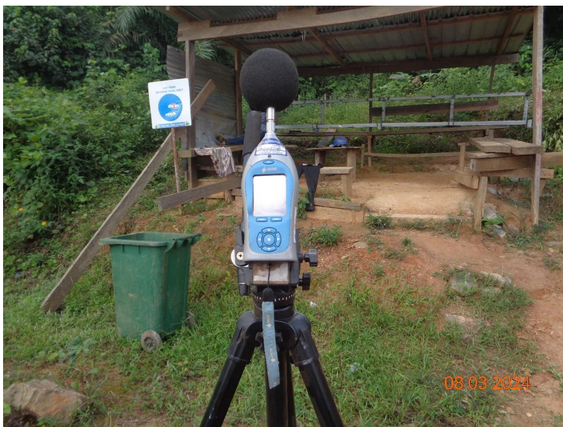
Plate 4: The Noise Monitor Positioned at AN1 (Apinto Mining Site)
