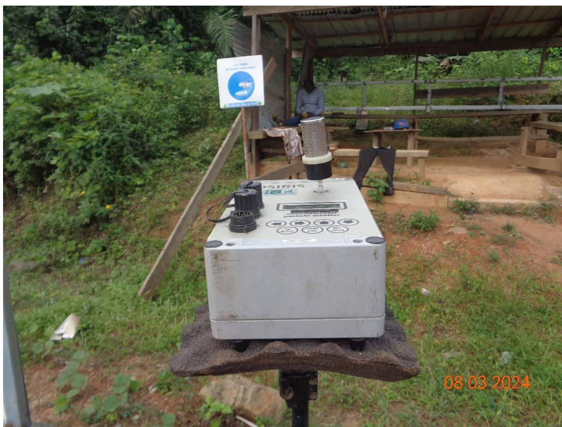
Plate 2: The Osiris Particulates Monitor at Location AN1 (Apinto Mine Site)
