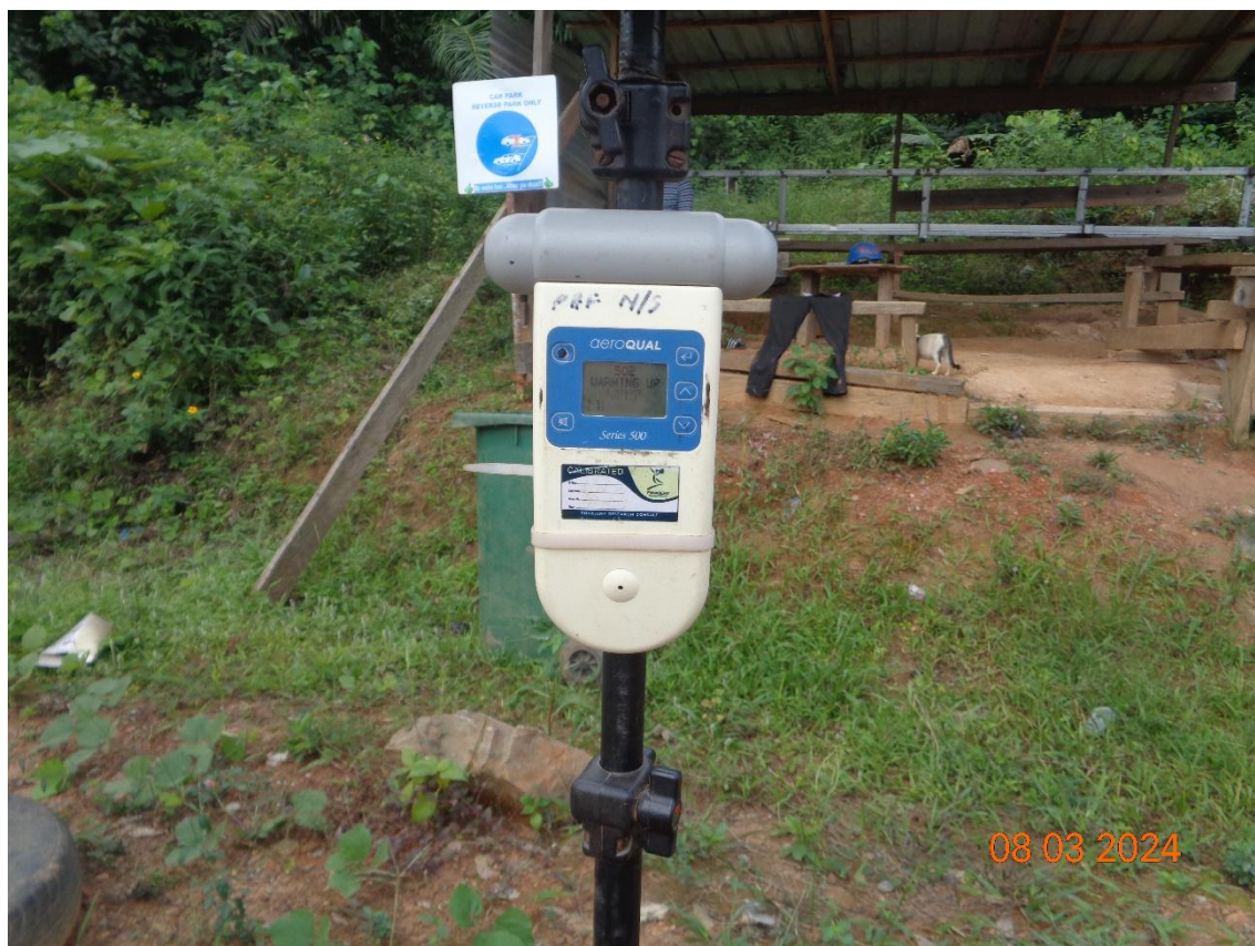
Plate 3: The Aeroqual Series 500 Gas Monitoring Deployed at AN1 (Apinto Mining Site)
